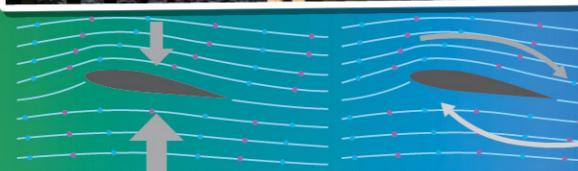
The faster moving air above the wing creates less pressure pushing down than there is pushing up.
